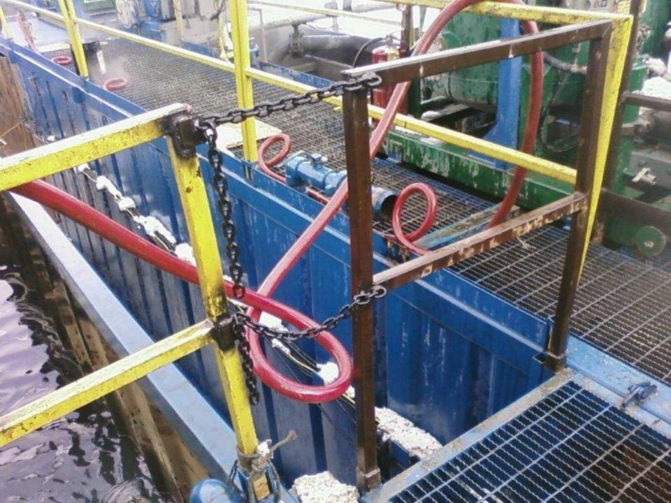
a floor hole that can cause a trip; materials can fall through and strike a worker below
